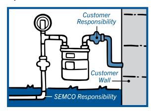
All equipment from the underground piping up to and including your gas meter, as indicated in the diagram, is SEMCO property and is serviced and maintained only by SEMCO Service Technicians or contractors. Customer-owned gas lines and connections between the outlet of the meter and your home, as indicated in the diagram, are the responsibility of the homeowner and should be serviced by a qualified plumber or heating and cooling specialist.
